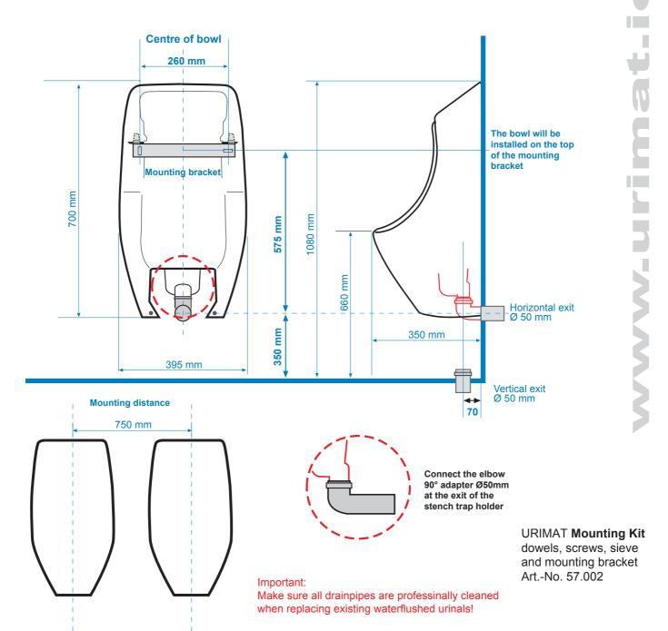
IMPORTANT: EU-Standard min. downgrade for wastewater pipes = 2%, i.e. 2cm per metre drainpipe, ideally 3%, but 5% maximum!
