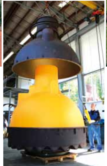
Rainwater storage tank production
