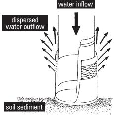
The smoothing inlet (EB 0300) acts as a brake and slows the incoming water down. The construction provides at the same time a calmed, dispersed water outflow upwards into the storage. By this it prevents stirring up the soil sediment of the storage and distributes the fresh rainwater.
