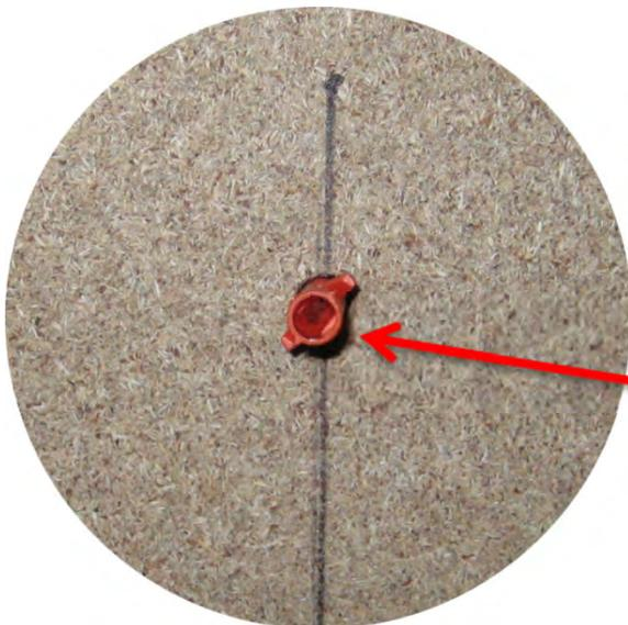
Insert a dowel into the drilled holes
