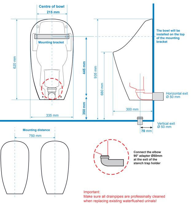
IMPORTANT: EU-Standard min. downgrade for wastewater pipes = 2%, i.e. 2cm per metre drainpipe, ideally 3%, but 5% maximum!
