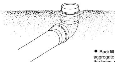
Backfill the waste pipe trench with appropriate compacted aggregate as normal, leaving the end of the 90-degree bend with the bung protruding.
