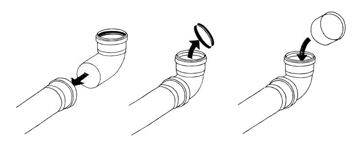
• The pipe that will carry the waste water to drain connects to the outlet beneath the unit. This pipe must have a 90-degree bend attached in order to meet the filter outlet. The pipe bung should be inserted in the open end of the 90-degree bend, having first removed the rubber seal. The bung will prevent debris from falling into the pipe during the installation process.
