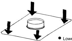
• Lower the steel base plate over the end of the pipe and position it dead flat on to the sand base. Ensure that the base plate is completely flat and that there are no cavities beneath it.
