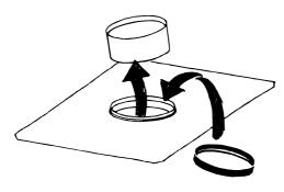
• Remove the pipe bung and insert the rubber seal removed earlier back into its position.
