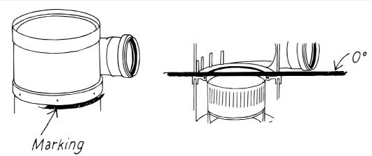
• Having aligned the filter correctly, the two halves of the unit must now be checked to ensure that they meet properly. This is when the mark below the upper housing ring is visible to exactly the same extent all the way around the unit.
