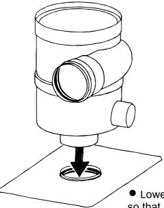
• Lower the WFF300 unit carefully over the end of the pipe so that it rests flat and evenly on the base plate
