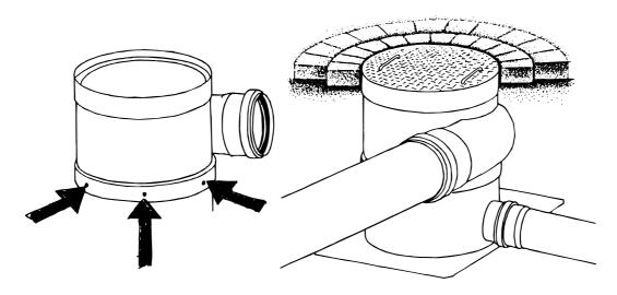
• Refit the retaining screws to secure the two halves of the filter. Connect the rainwater inlet pipe and the clean water outlet pipe to the filter. The WFF300 filter is now ready for use.
