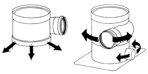
• Align the rainwater inlet and the clean water outlets of the filter to face the desired directions to meet the relevant pipework. To achieve this, first unscrew the retaining screws from the 'waist' of the unit where the top ring overlaps the bottom.
